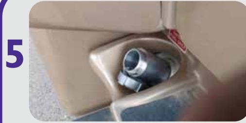
**5** Ensure cap retaining chain measures three and a half inches as illustrated (if too short see below)
