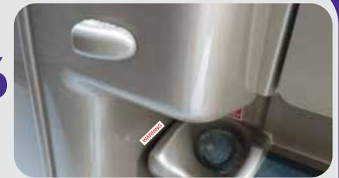
**6** Install **warning** label in location that is visible when filling tanks
