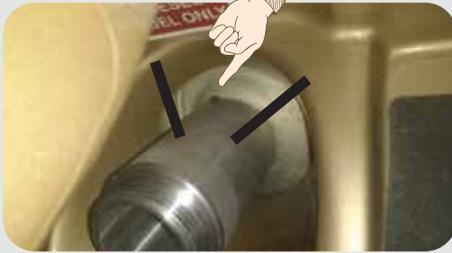
**4** Start and thread extension on and position Allen lock screw towards top (to ease tightening of locking screw)
