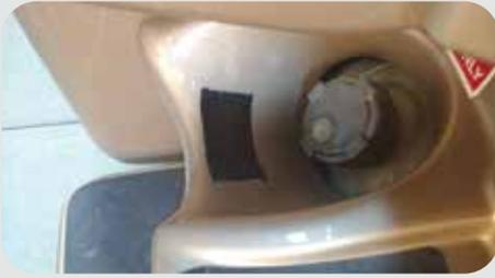
**1** Install protective wrap (to prevent fuel cap scuffing). Size and shape may be different than illustrated
