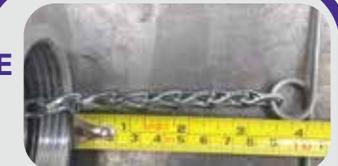
**E** Install safety T on other end and screw fuel cap onto extension
