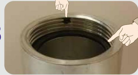
**3** Ensure locking Allen set screw not protruding into threads for ease of assembly
