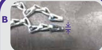
**B** Due to factory pin heights a small amount of eye loop may have to be removed (grinder or file)
