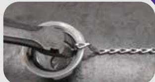
**A** Using side cutters cut factory chain
