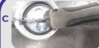
**C** Open eye and install over factory pin, pinch eye shut allowing movement of chain around stud
